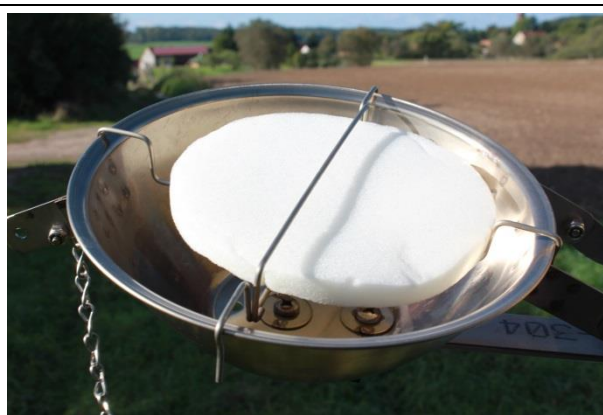
Abb. 16: Sammelmedium Sorbent Impregnated Polyurethane Foam Disk (SIP)
